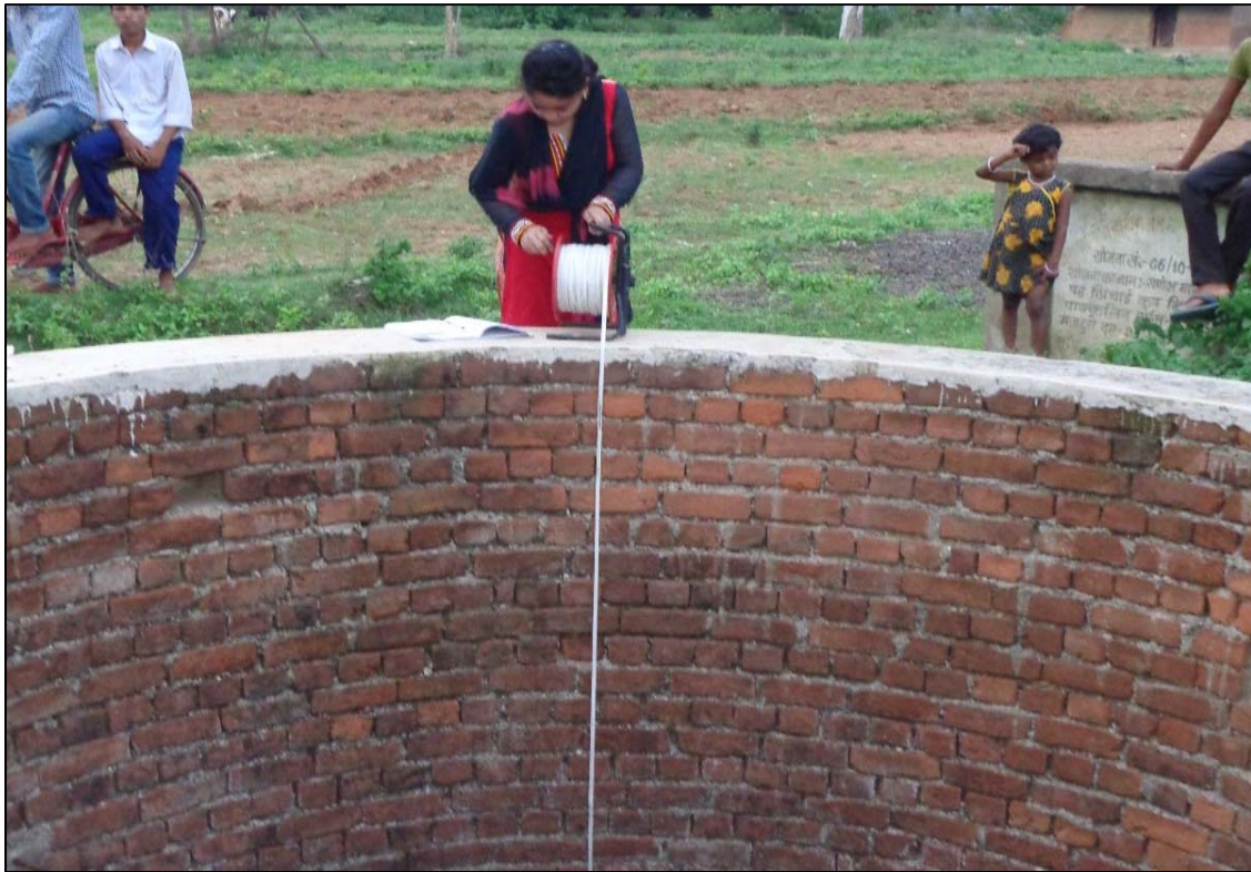
Figure 3. Infiltration Test in Musabani Block (2015)
