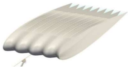
Fig. 1: Proposed new design of a quiet aerofoil of the next generation
