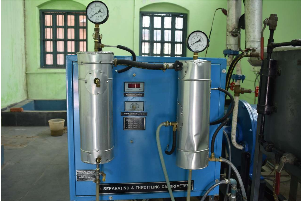
Fig. 2 Photograph of separating and throttling calorimeter
