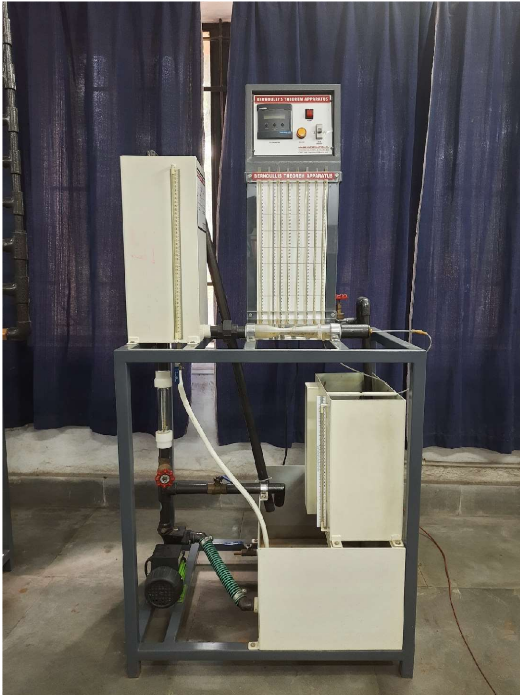
Fig. 1.2 Experiment setup of Bernoulli's theorem
