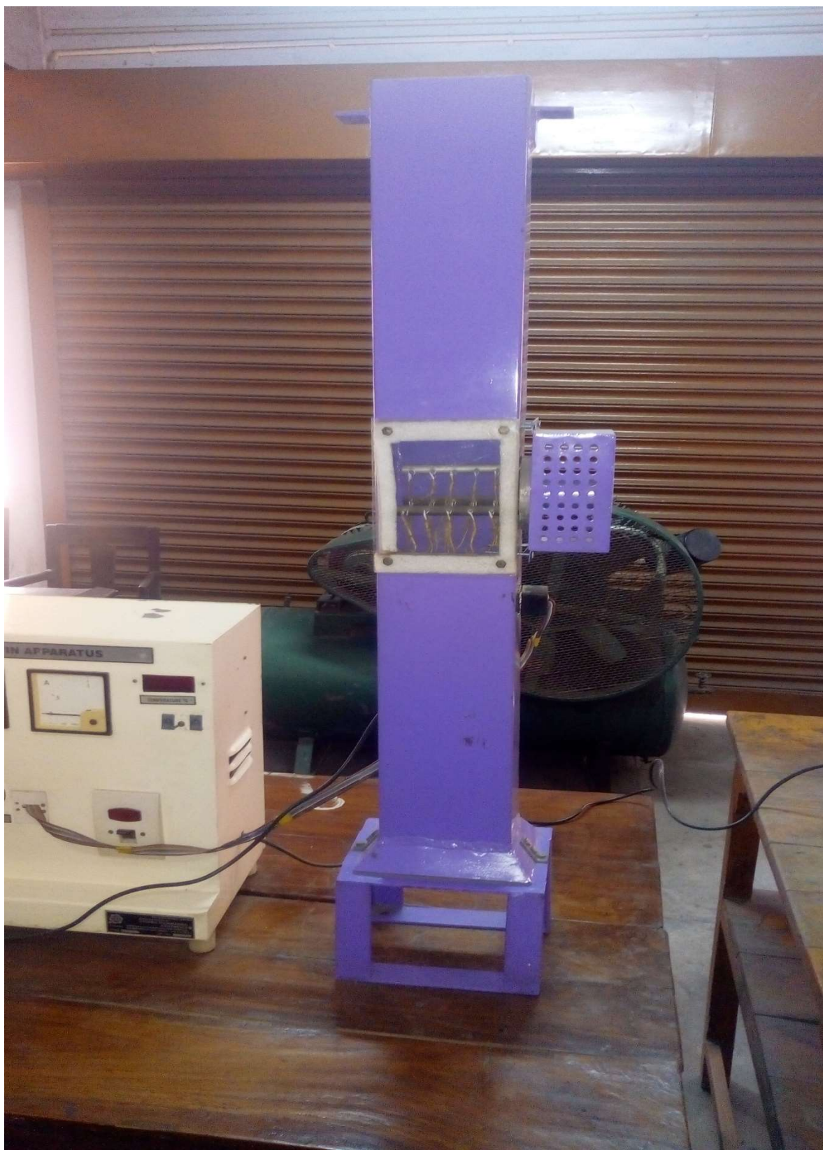
Fig. 1 Experimental setup of Pin-fin apparatus
