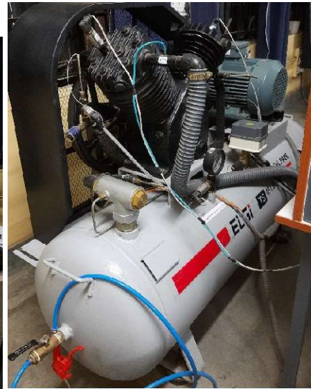
Fig. 6.3 Experiment setup of 2 stage reciprocating air compressor test rig
