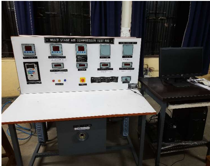
Fig. 6.3 Experiment setup of 2 stage reciprocating air compressor test rig
