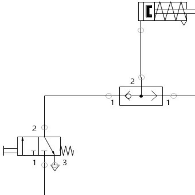
**Fig:** Pneumatic Circuit Diagram of OR Circuit.
