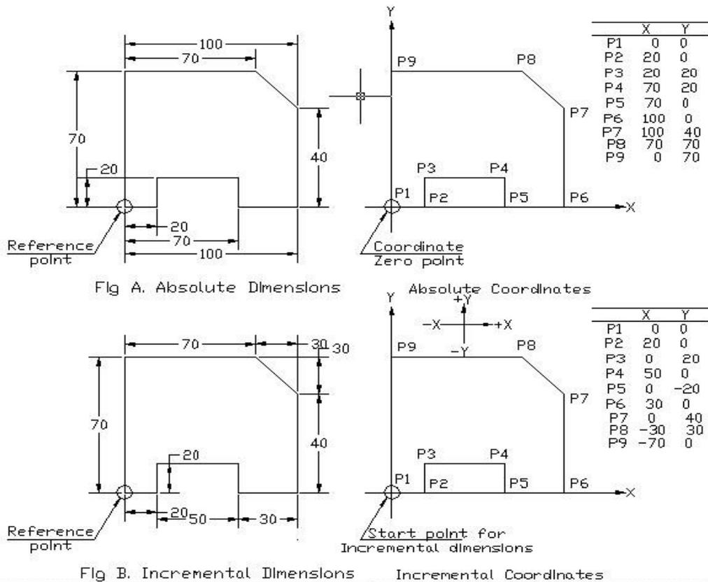
**Observation:** Write a CNC part program for the following milling operation.
