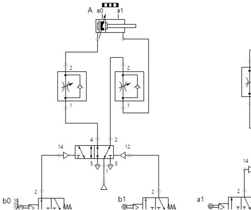
**Fig:** Pneumatic Circuit Diagram for sequences such as A+ B+ A- B-
