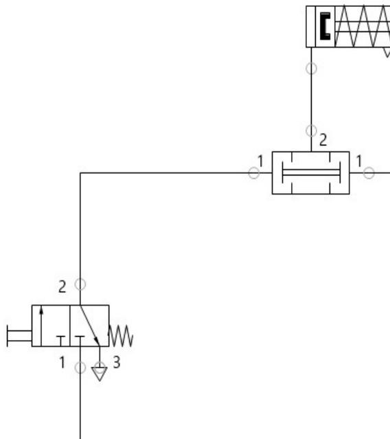
**Fig:** Pneumatic Circuit Diagram of AND Circuit.
