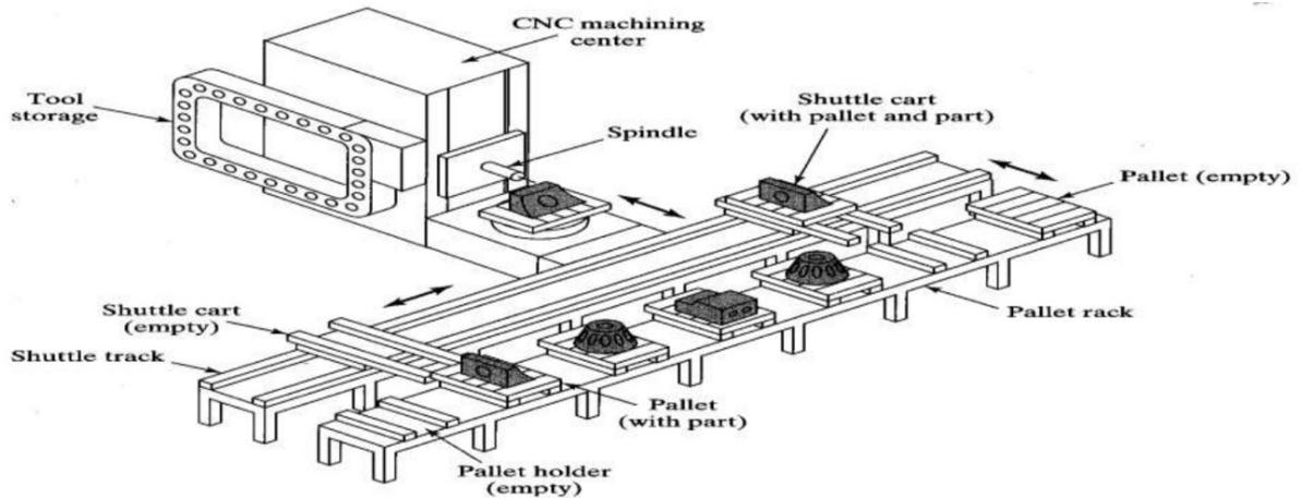
**2. Flexible Manufacturing Cell (FMC):** It entails two or three dispensing workstations and a material handling system. The material handling system is linked to a load/unload station.
