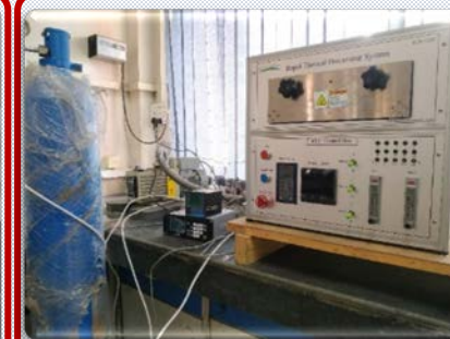
Rapid Thermal Processor (Rising rate (max) 80°C/sec., Temp: up-to 1200 °C Under controlled gaseous environment) (Make: Ecopia RTP 1300)
