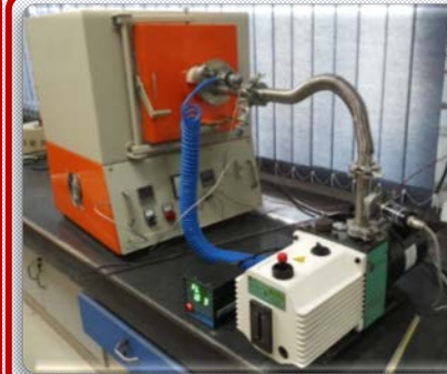
Muffle Cum Tube Furnace (Rising rate up to 15°C/min, Temp: up-to 1200°C Under controlled gaseous environment) (Make: Ants Innovations (P) Ltd)
