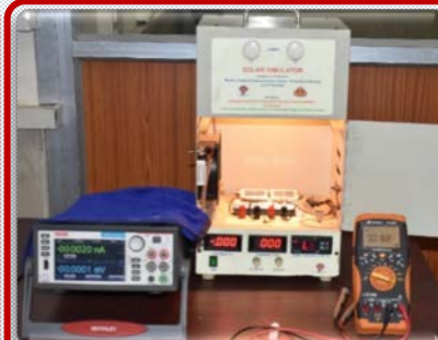
Solar Simulator & SMU Make: NCPRE, IIT Mumbai & Keithley
