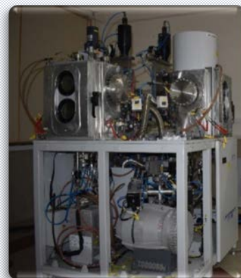
Customized Dual Chamber PVD System for Thin Film Deposition [RF/DC Sputtering (3 confocal magnetron), Thermal, and E-beam Evaporation] Make: HHV Pvt. Co. Ltd.
