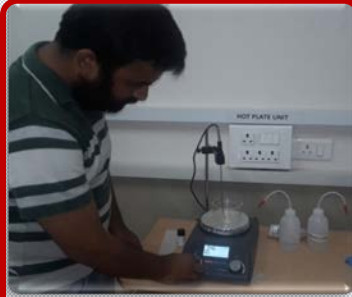
Hot plate with magnetic stirrer (temp up to 350°C) Make: REMI
