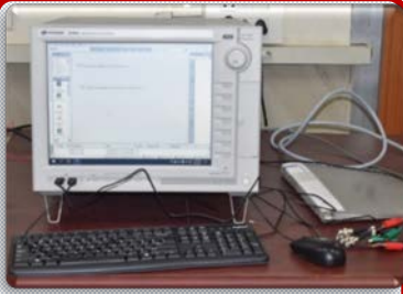
Semiconductor Parameter Analyzer (with I-V, C-V, C-F) Make: KEYSIGHT B1500A
