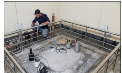
Broadband, Analog and Short Period sensors installed on a concrete pillar
