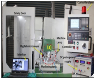
Hybrid Micro Machining Technology using \mu -ECM and \mu -EDM Processes
