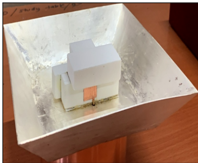
High Power Handling Dielectric Resonator Antenna
