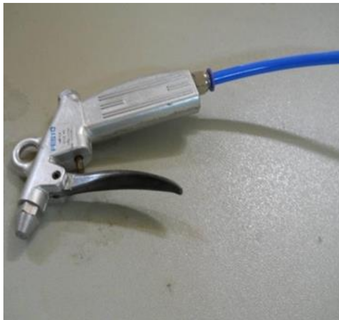
Fig. Compress air blower
