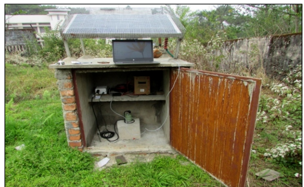
Broadband Seismometer Installed at Peterbar (Jharkhand)
