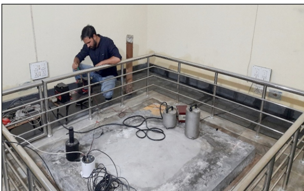
Broadband, Analog and Short Period sensors installed on a concrete pillar
