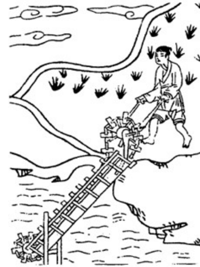
Dragon backbones (a) hand-operated; (b) foot operated
