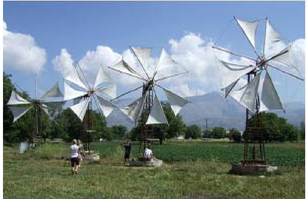
Water pumping sail-wing machines in the plateau of Lassithi in the Island of Crete
