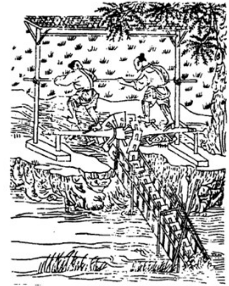
Dragon backbones (a) hand-operated; (b) foot operated
