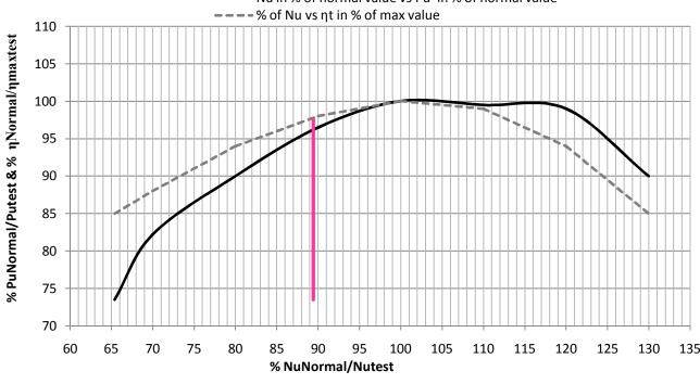
Normal unit power  $P_{uNormal}$  = 74.9 kW/m^1.5 normal efficiency  $\eta_{normal}$  = 90.6 %
