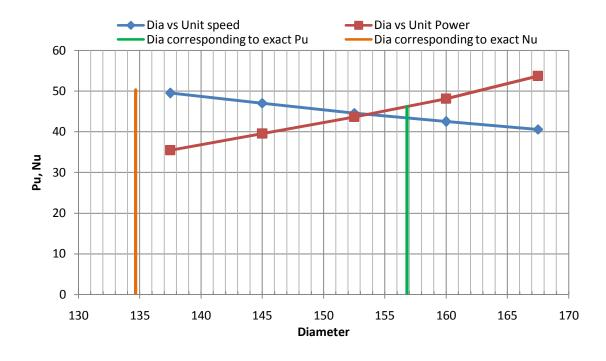
for the above unit power (Pu) diameter of the runner can be calculated from the above table
