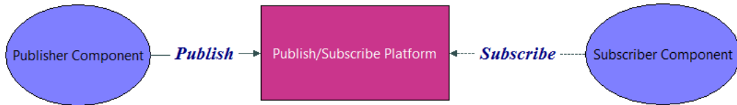
Figure 6.1: Example showing: Components, Pub/Sub Platform, Publish and Subscribe Connections
