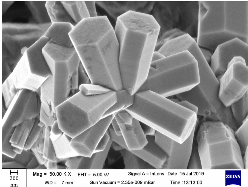
Figure 3.7: The grown ZnO NSs under processing condition of 90°C, 4h, 6.5pH and 10mM
